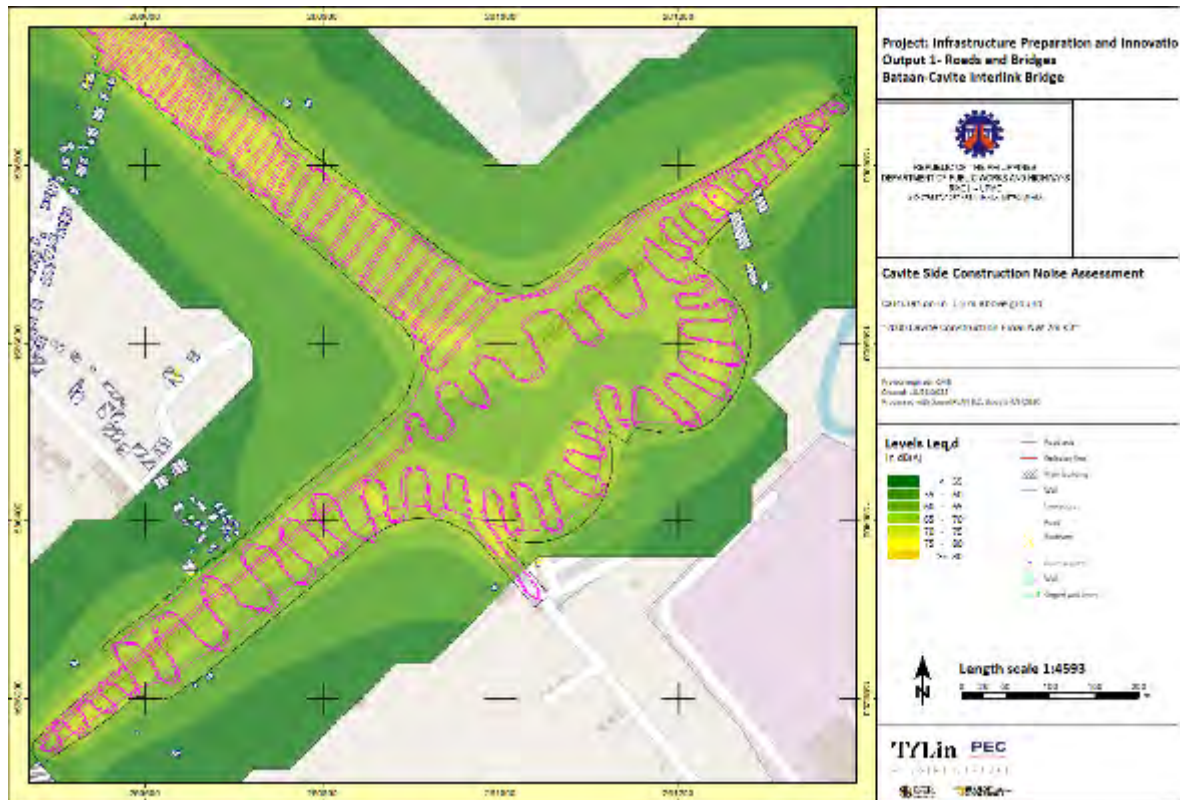
Figure A8. Section 2 Cavite Construction Noise Contour Map Daytime 2m Noise Walls
