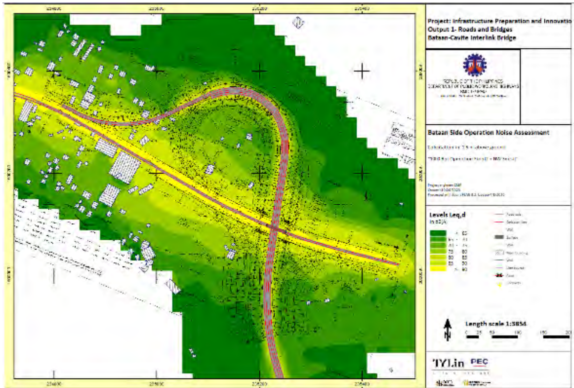
Figure A14. Section 1 Bataan Operational Noise Contour Map Day time 3m Noise Walls
