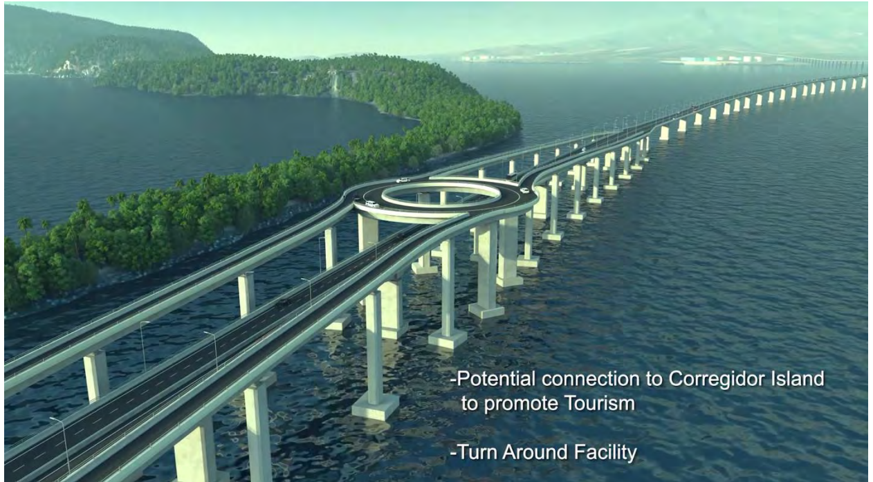
Proposed mid-span turnaround, with possibility of connection to Corregidor Island in future
