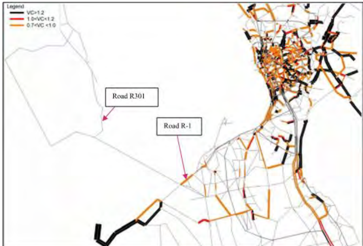
Exhibit 1-68: Network Performance in V/C ratio for 2025 AM "with project" case
