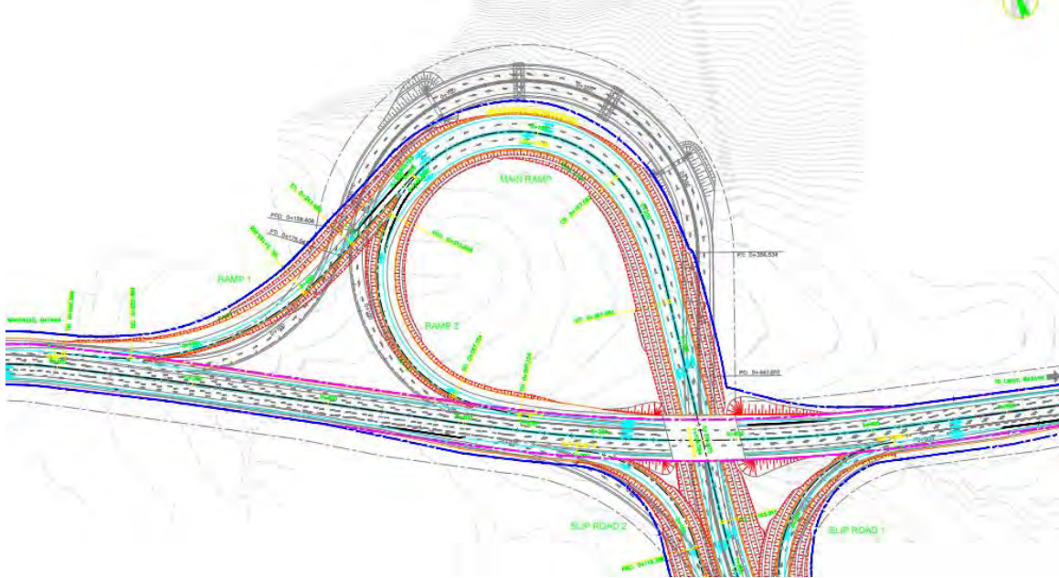
Exhibit 7-19: Overlay of the FS Alignment (grey) and the Optimized Alignment (colored)
