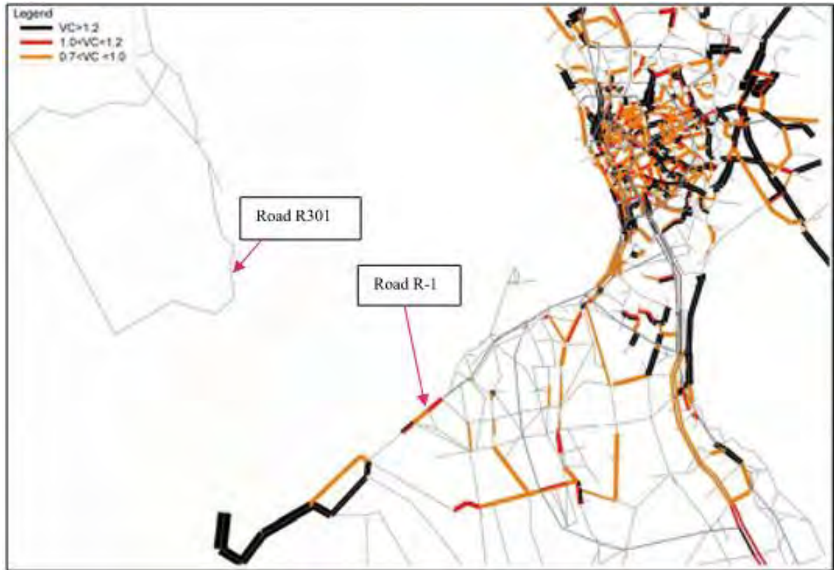
Exhibit 1-67: Network Performance in V/C ratio for 2025 AM "without project" case
