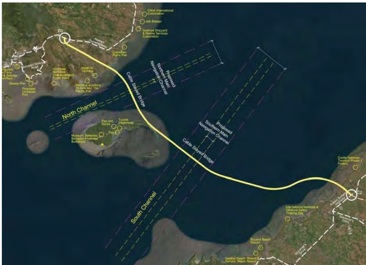
Exhibit 1 Plan View of BCIB Showing Navigation Channels
