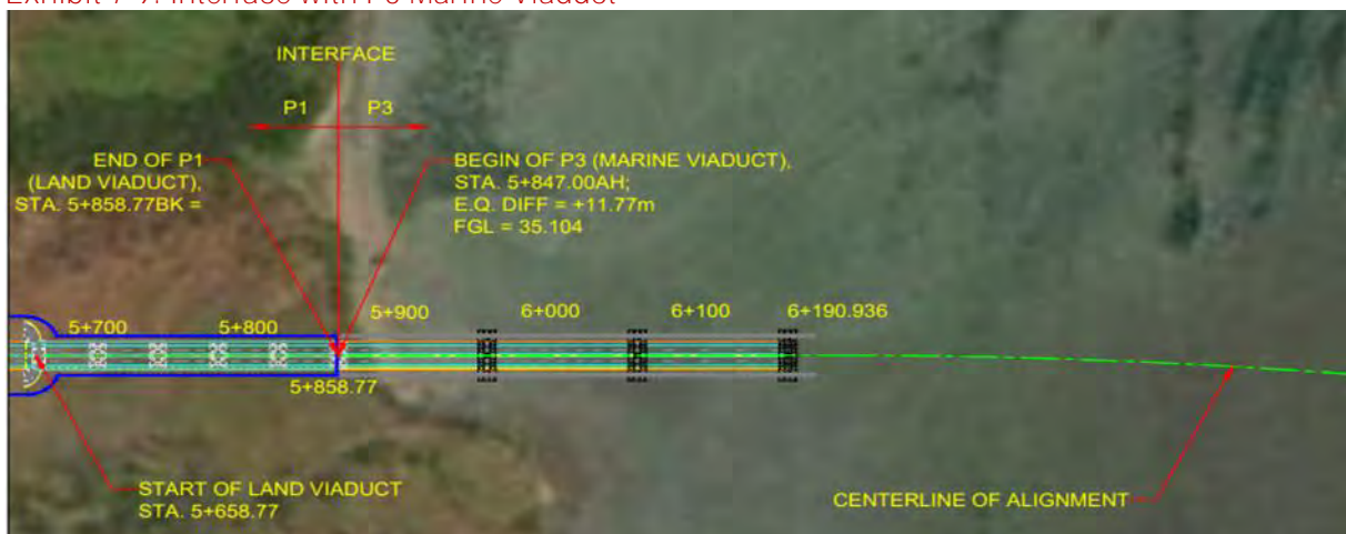
Exhibit 7-9: Interface with P3 Marine Viaduct
