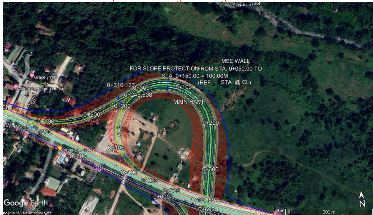
Exhibit 5-24: Landslide Susceptible Areas Along Bataan Alignment
