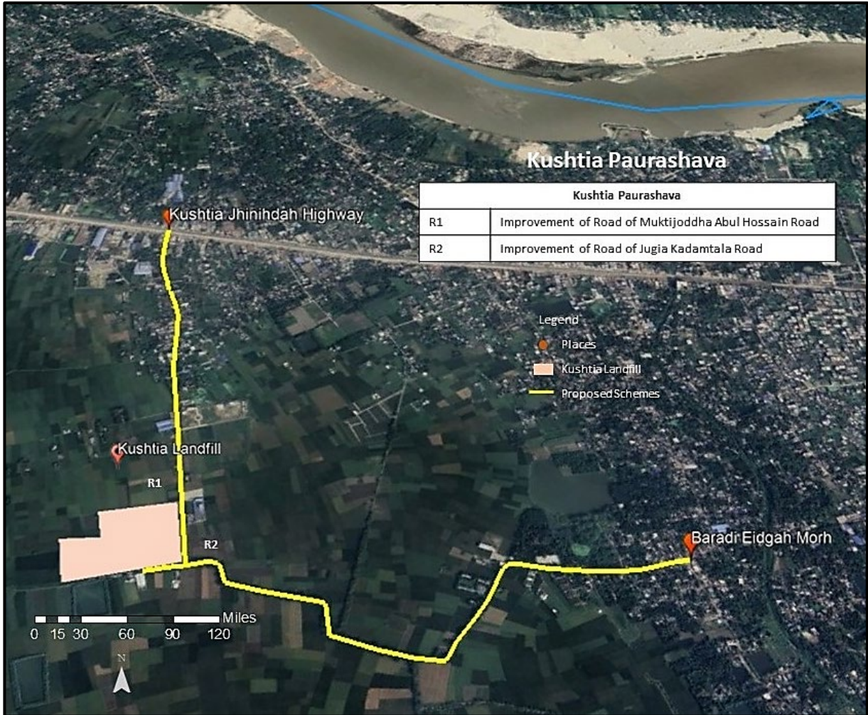
Figure 3: Location and Alignment of the Connecting Roads Proposed for Improvement for the Landfill Site
